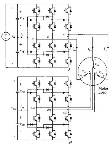
Fig. 4. Cascade-3/3 multilevel inverter.
